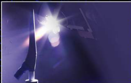
ROBOTIC PLASMA SPRAY COATING FOR MEDICAL IMPLANTS
