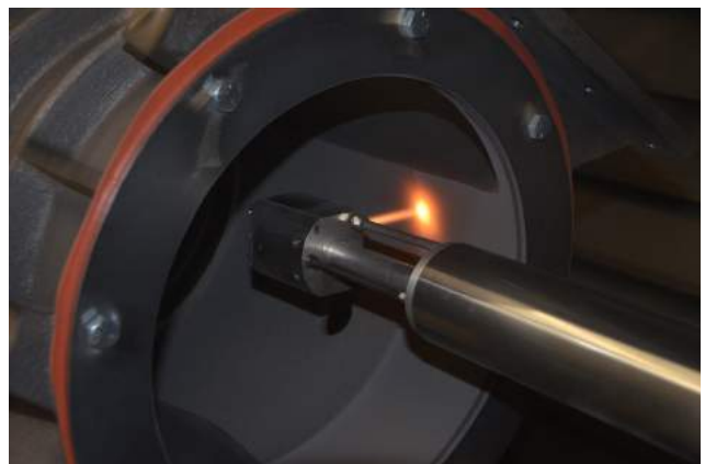
Fig. 2 — UniqueCoat's I7 torch coating the internals of a rotary valve.
