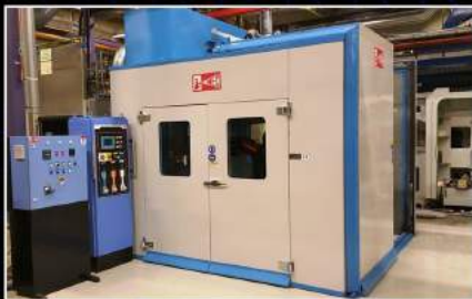
7 AXES ROBOTIC FLAME SPRAY COATING
