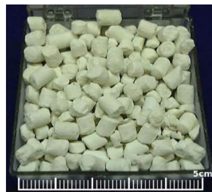
Lithium pellets. To be used as a raw material for batteries, lithium must be at least 99.5% pure.
