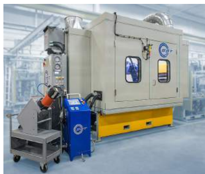
Fig. 1 — Commercial downstream injection cold spray system. Courtesy of CenterLine Windsor Ltd.
