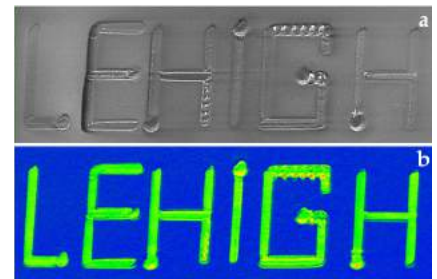
Scanning electron micrograph (a) and image quality map (b) of the micrograph demonstrate the ability to fabricate patterned single-crystal architecture on a glass surface. Courtesy of Dmytro Savvtskii.
