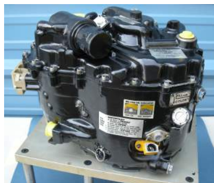
Fig. 2 — Boeing 747 integrated drive generator (IDG). Courtesy of L.J. Walch.
