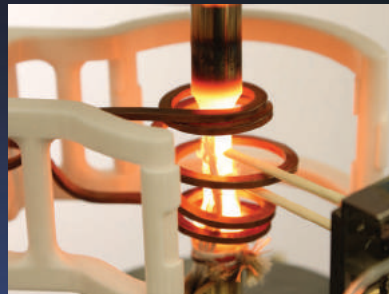
MTS Thermomechanical Fatigue (TMF) testing solutions supports temperatures up to 1200 °C
