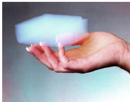
Fig. 3 — Aerogel foam for capturing cosmic dust.
