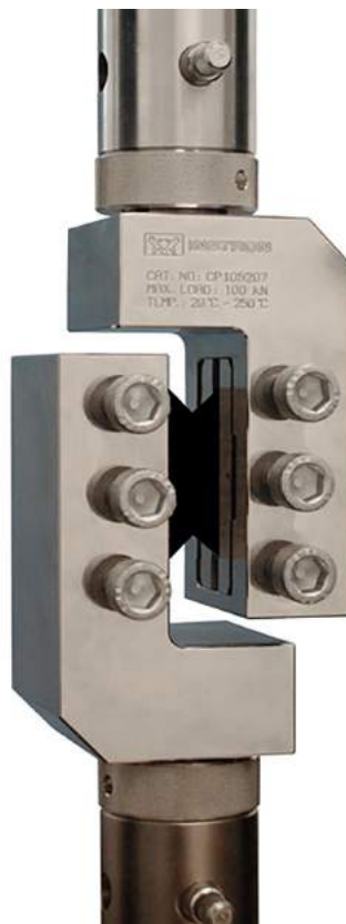
ASTM D7078 V-notched shear specimen and test fixture.
