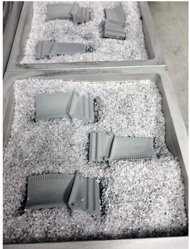
Fig. 1 — Test turbine engine blades produced by the EBAM process.
