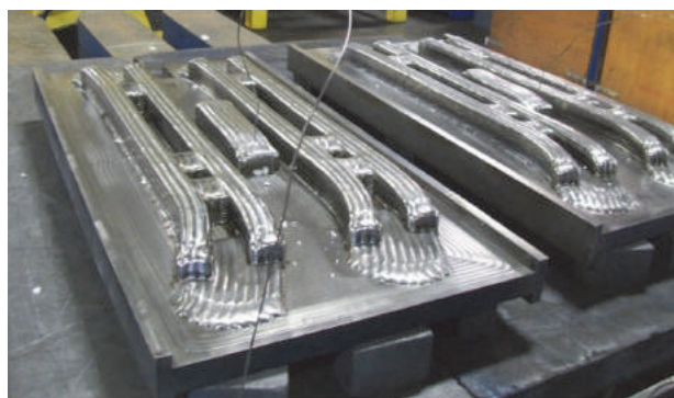
Fig. 3 — EBAM is used to deposit titanium wire on a titanium base.
