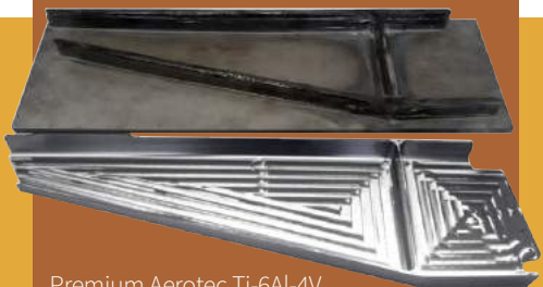
Premium Aerotec Ti-6Al-4V sample part additively manufactured by Norsk Titanium. Courtesy of Business Wire.
