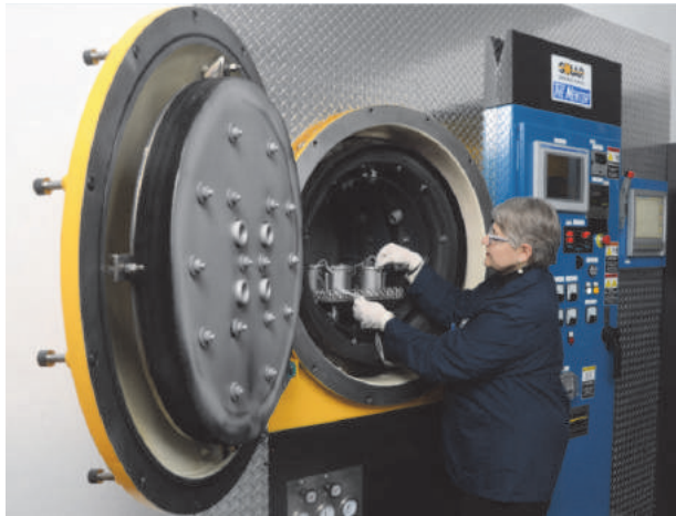
Fig. 5 — AM-capable vacuum furnaces range from lab size to 48 ft long.
